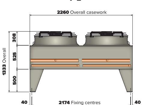
**Note:** All dimensions in mm. Common junction box will vary in size and position depending on the control option required.
