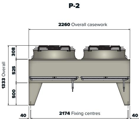
**Note:** All dimensions in mm. Common junction box will vary in size and position depending on the control option required.
