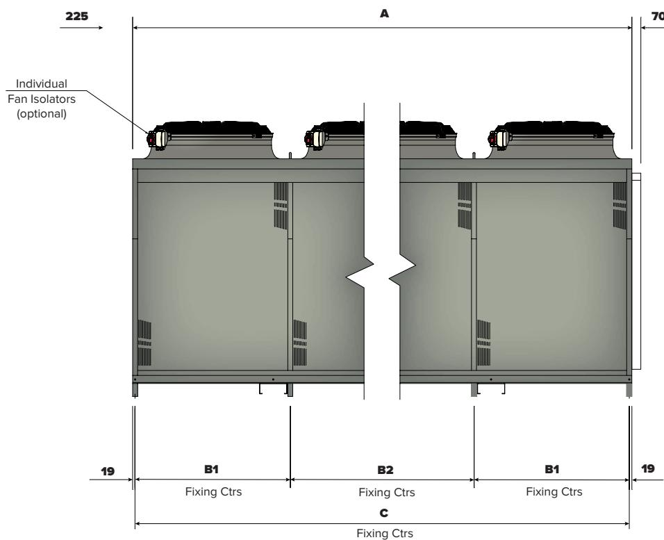
**Note:** All dimensions in mm. Common junction box will vary in size and position depending on the control option required.
